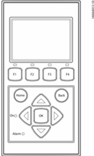
Figure 3.1 Overview of display buttons and functionality
