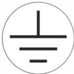
Figure 2.19 Protective conductor symbol
