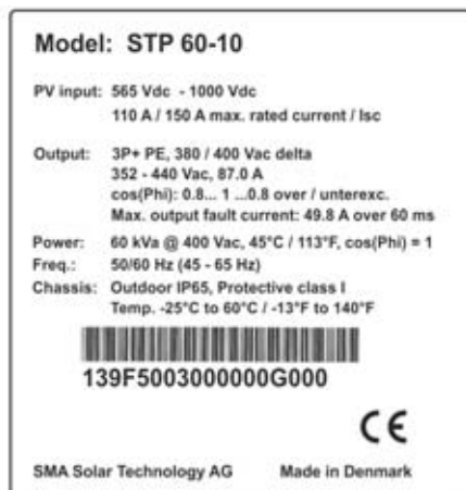
Figura 1.3 targhetta Sunny Tripower 60
