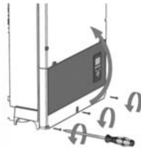
Figure 2.15 Loosen front screws and lift the cover
