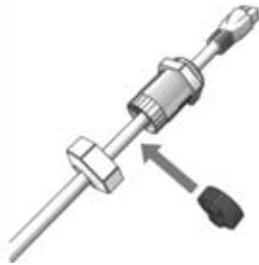
Figure 2.22 Run cables through cable glands
