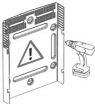
Figure 2.10 : Montage du support mural
