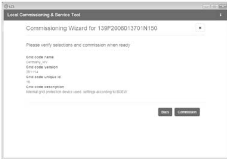
Figure 3.8 LCS tool - Verification of country and grid code
